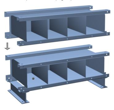
step 5: Install the 3rd, 4th,5th layer...on the lower modular frame until all modular frames are aligned and installed.
