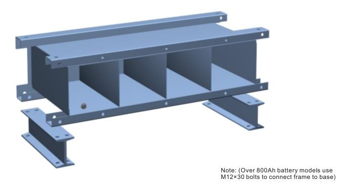
step 3: Move the modular rack assembly to the final position and mark hole locations. Next move the rack and drill anchors holes at the marked locations. Follow 1) user supplied anchor mounting instructions or 2) move rack back to the final position, install M10 expansion bolt anchors into the holes and tighten the nut to secure the rack to the floor.
