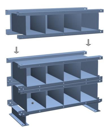
step 6: The cell layout and connection diagram will be supplied with the original quote, the rack or is available on www.sbsbattery.com. Orientate cells per drawing. Pay attention to the polarity of the cells. Install hold down bars after cells are mounted.
