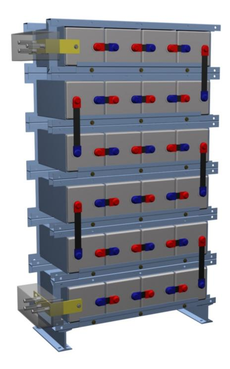
step 8: Install the standoffs and Plexiglas shields (covers) to the modular frame from the bottom up.
