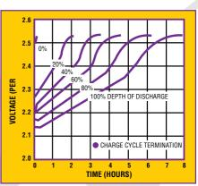
Should the user prefer a voltage/time charge termination, the AC1000 can be set for this popular termination method through available programming options.
