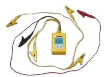
During capacity testing, the wireless modules measure each cell's voltage and wirelessly send the data back to the paired load bank. All voltage values are displayed on the load bank's LCD screen and listed in the test report, which is created with the computer software. Wireless modules make it easy to locate failed or problematic cells in the battery bank.
