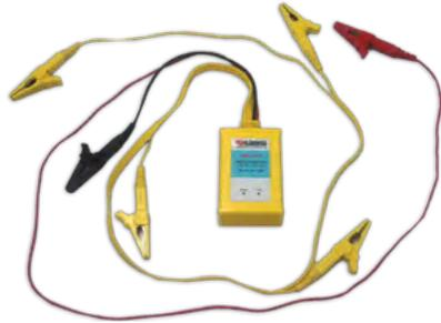
During capacity testing, the wireless modules measure each cell's voltage and wirelessly send the data back to the paired load bank. All voltage values are displayed on the load bank's LCD screen and listed in the test report, which is created with the computer software. Wireless modules make it easy to locate failed or problematic cells in the battery bank.
