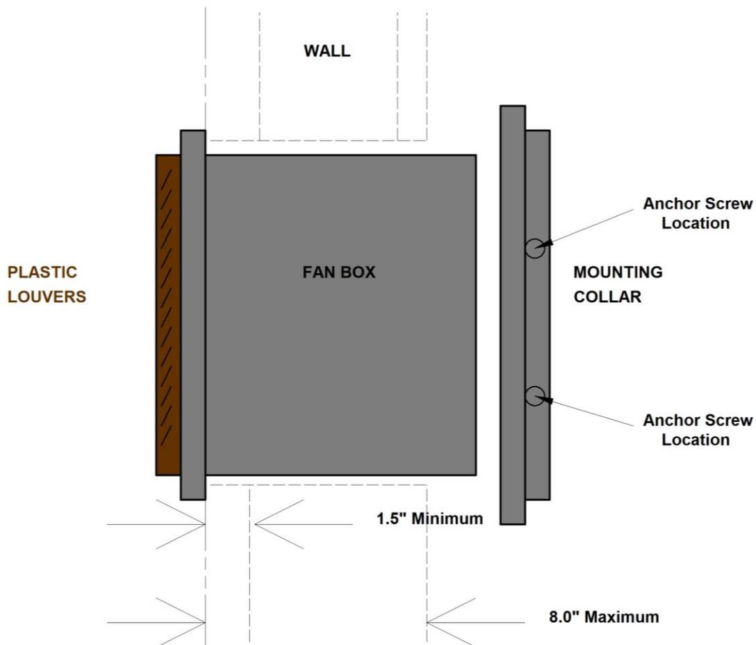
*(mechanical bracing or duct transition inserts can be used to achieve minimum wall thickness)*
