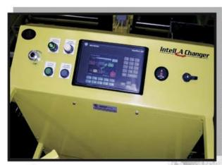
The "brain center" of the Intell-A-Changer: the Allen-Bradley ControlLogix PLC.
