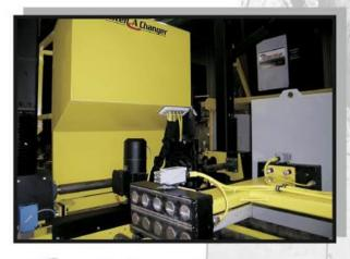
The T-arm utilizes a worm gear electric drive to transfer the magnet from one side to the other.
