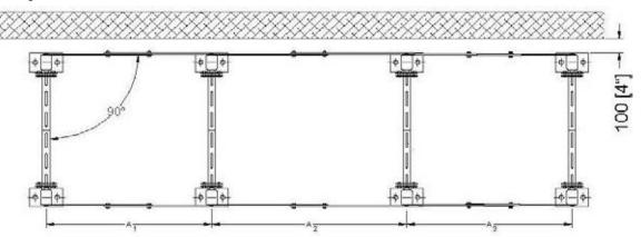
If an SBS **spill containment system** is supplied the rack will be installed inside the polypropylene spill pans. Polypropylene is acid resistant, extremely strong and can support up to 15,000 lbs. per square inch without degradation of the material. SBS supplies different size spill pans that are butted together in different combinations to form different spill containment system lengths and widths. Flexible connectors are supplied to 'connect' the pans together.
