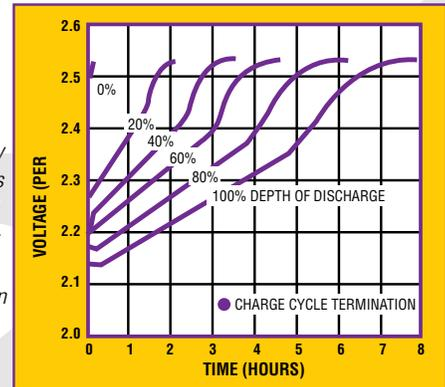
Should the user prefer a voltage/time charge termination, the AC1000 can be set for this popular termination method through available programming options.
