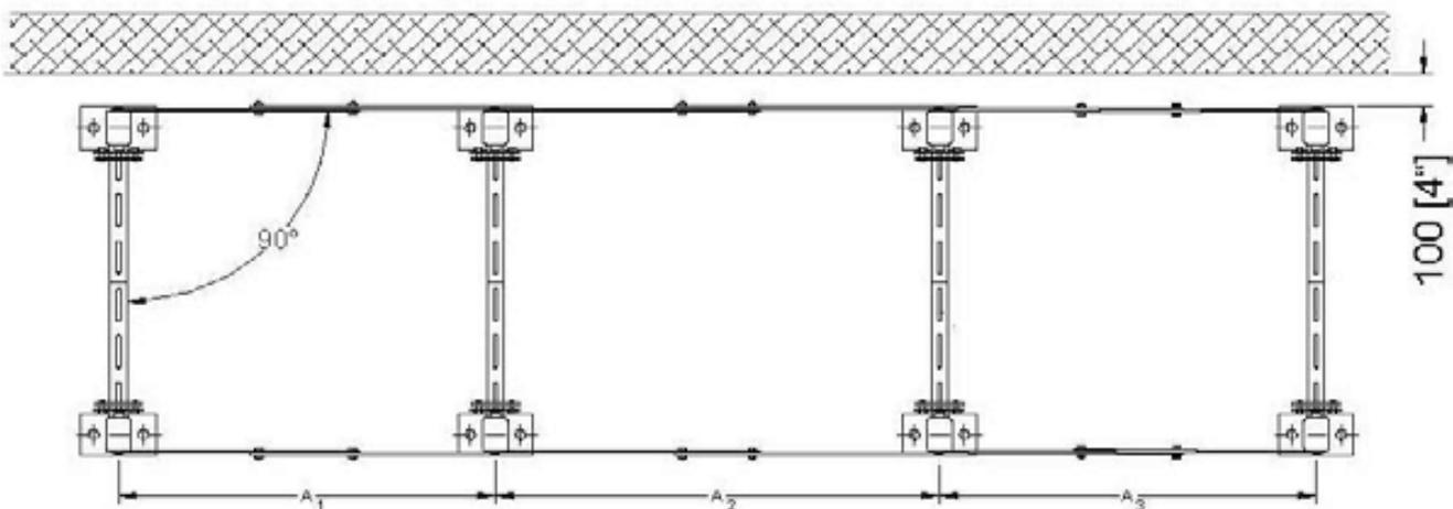
If an SBS **Spill Containment System** is supplied the rack will be installed inside the polypropylene spill pans. Polypropylene is acid resistant, extremely strong and can support up to 15,000 lbs. per square inch without degradation of the material. SBS supplies different size spill pans that are 'butted' together in different combinations to form different spill containment system lengths and widths. Flexible connectors are supplied to 'connect' the pans together.
