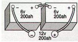
**Figure 1:** These are two 6 Volt batteries in series to produce 12 Volts. You can add more batteries for a higher voltage, i.e. 24, 48, 130 Vdc.
