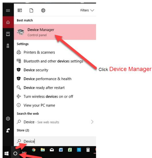
11. Windows will assign two (2) COM Port numbers. Try the 1<sup>st</sup> number and if you are unable to receive the SBS-2003 data then try the 2<sup>nd</sup> number. The SBS-2003-Data-Capture Excel workbook will only work with COM Ports 1-9. If Windows assigns a higher number you must manually change it. Once you know the two numbers close the Device Manager.
