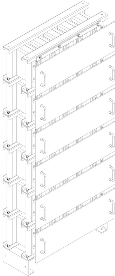
Note: Shields are not required. The AGM rack systems are provided with insulated intercell connector cables so protection is already in place.
